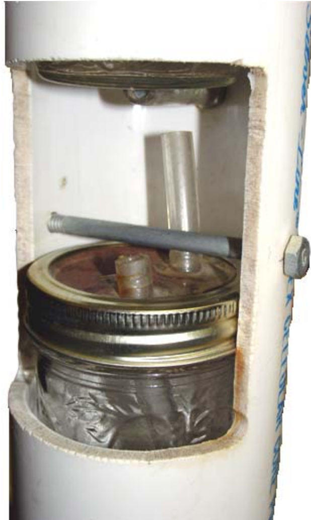
Figure 4.2. Rising stage sampler. (Photograph by the author.)
